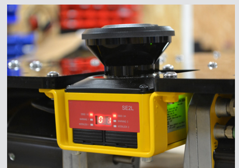
SIL2 / PLD safety scanner Compatible with all safety laser scanners on the market
