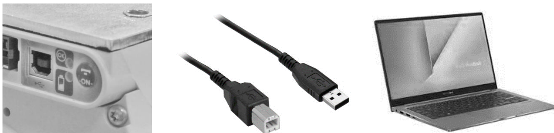
Figure 1 - Plug the USB-B cable to the back port of the wheel Connect the USB-A cable to the wheel
